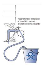
Did you know that any connection between a public drinking water system and a separate source of questionable quality is considered a cross-connection? For example, an ordinary garden hose submerged in a bucket of water, car radiator, or swimming pool can result in backflow contamination. To protect our water supply, a simple screw-on vacuum breaker must always be attached to the faucet when a garden hose is used. In addition garden hoses must be detached from faucets when not in use.
